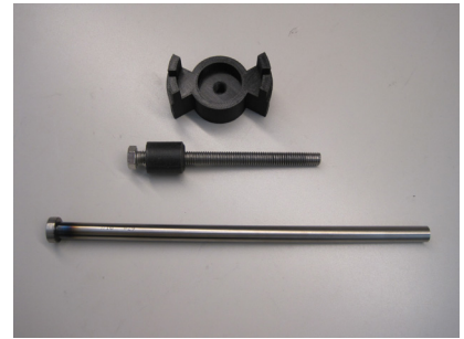
Fig 24: Impeller Removal Tool includes: prong release tool, 5" long bolt, bushing, & drive pin.
