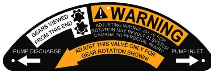
DIRECTION OF ROTATION TAG FOUND ON 3632 – 3748 BV STYLE BI-DIRECTION RELIEF VALVES
