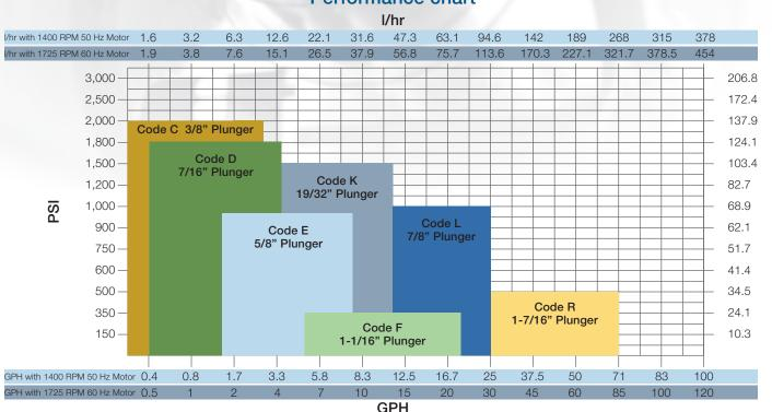
\*Values are for simplex pumps only. For duplex configurations, the pressure will not change, but the capacity values will double.
