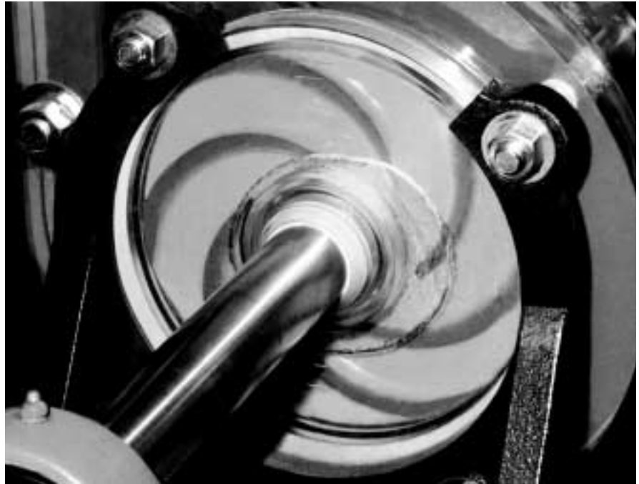
Wilfley hydraulic seal in actual operation.
