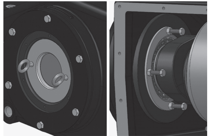
Crankshaft Alignment Donut Crankshaft Installation Bar
