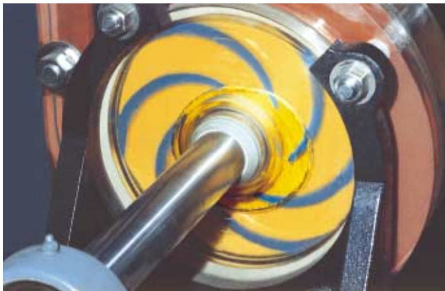
Wilfley hydraulic seal in actual operation.
