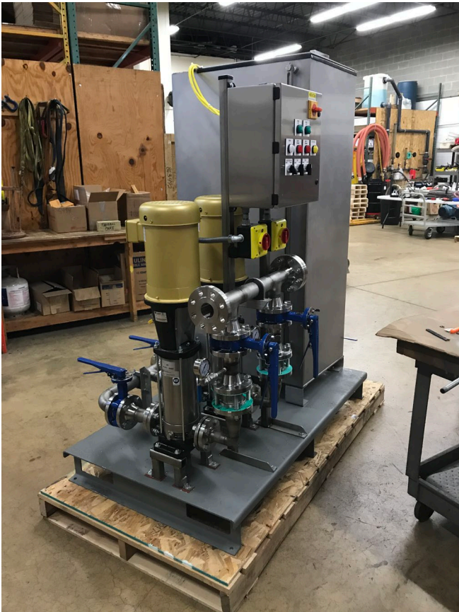
Water reclamation system with two Ebara® EVMSU vertical multistage pumps, fabricated stainless steel tank with level controls, control panel with disconnects, mounted to a fabricated steel base plate to fit through a customer-specified door entrance
