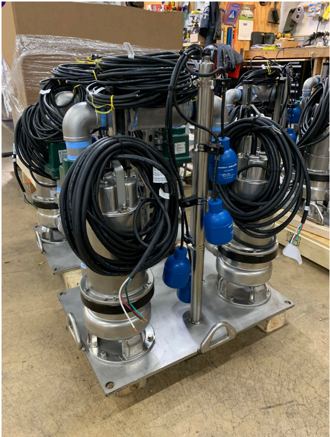
Sump pump package with two Ebara® Dominator stainless steel submersible sewage pumps, fabricated steel mounting/lifting plate, and float switches for drop-in installation in a drainage sump
