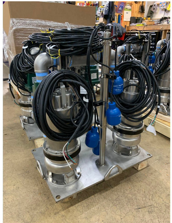
Sump pump package with two Ebara® Dominator stainless steel submersible sewage pumps, fabricated steel mounting/lifting plate, and float switches for drop-in installation in a drainage sump
