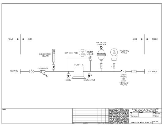
Pump Cube systems include with valves and accessories for simple installation, calibration, and verification of operation.
