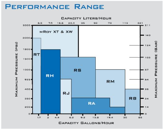
Milton Roy mRoy series pumps are available to 85 gallons per hour (170 gallons per hour for duplex pumps), with discharge pressures to 3000 PSI.
