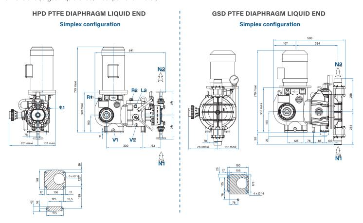
N1 Suction - N2 Discharge - V2 Drain hydraulic oil - L2 Hydraulic oil level - R2 Hydraulic oil filling - V1 Drain mechanic oil - R1 Mechanic oil filling - L1 Mechanic oil level
