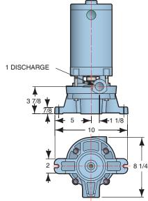
All dimensions are in inches. May vary ± 1/4 inches. Model M52 shown in Multistage Dimensions. Model M51 shown in Single Stage Dimensions.
