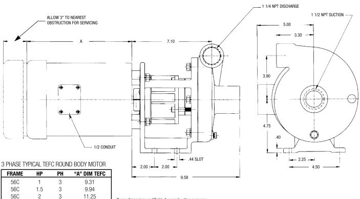
Pump dimensions certifiable for construction purposes. Motor dimensions dependent upon motor manufacturer.
