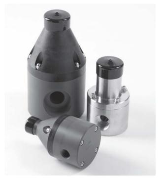
**Griffco G-Series** diaphragm back pressure valves are designed to enhance the performance of chemical feed systems by applying a continuous back pressure to the chemical feed pump, while also acting as an anti-syphon valve. Robust construction ensures reliability in the rigorous service of municipal and industrial applications. Wetted materials include: PVC, CPVC, PP, PVDF, PTFE, Halar, 316 SS, A20 and Hast. C. Available sizes: 1/2" – 4".
