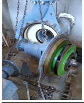
Back pull out structure enables disassembly and inspection without removal of suction and discharge piping.
