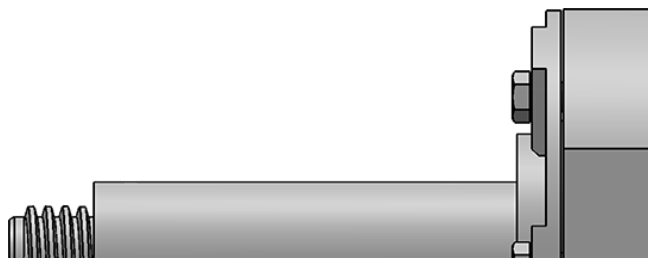
Incorrectly installed shaft sleeve (Shoulders against thrust bearing isolator o-ring)
