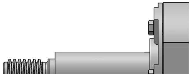
Correctly installed shaft sleeve (Shoulders against thrust bearing)
