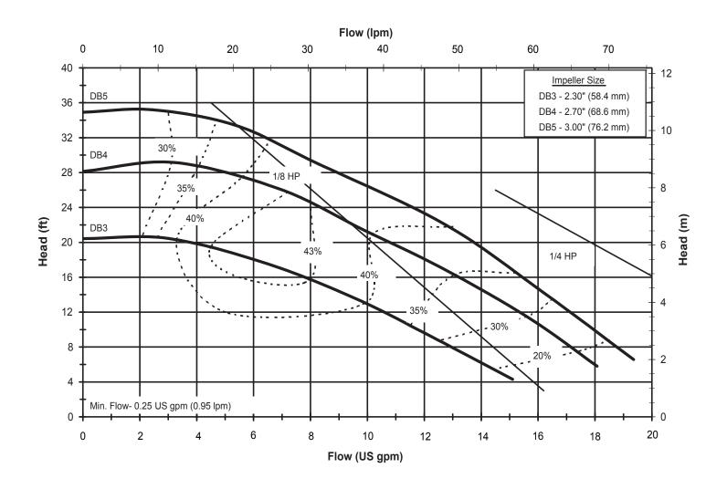
DB345-5060 6061 REV 0 Model DB3, 4, 5 2900 rpm, 50 Hz Suction: 1" FNPT Discharge: 1/2" MNPT
