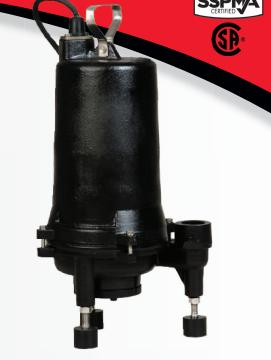
1 & 2 HP grinder pumps that have a 1 1/4" vertical discharge (optional 2" adapter available), and can grind up to 3" solids, and be installed on a rail system or with the supplied legs
