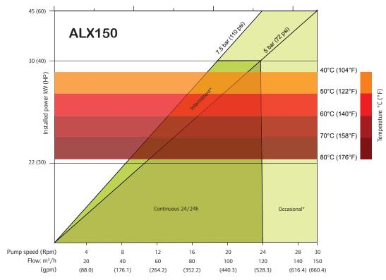
1 rpm = 5.000 m<sup>3</sup>/hr = 22.0143 gpm 1 rev = 83.3333 L = 22.0143 gal
