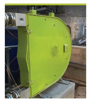
Displacing 83.33 litres (20 gallons) per revolution, you can run this pump very slowly to deliver high flow rates up to 150 m3/h (660 gpm) with excellent hose life.
