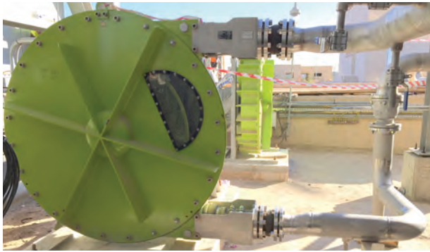
ALH125 pumping concrete
