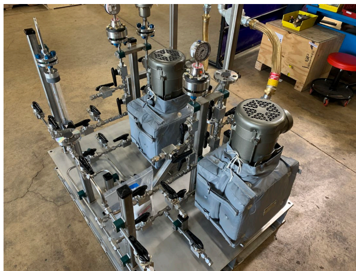
Chemical additive skid with two Milton Roy® mRoy™ series pumps, stainless steel tubing, explosion-proof motors and control panel, and custom-fit insulating pump jackets
