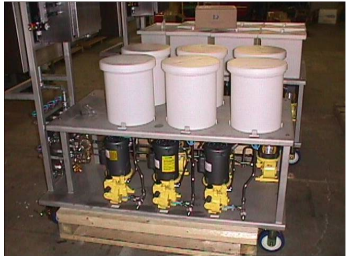
Food additive package with Milton Roy® mRoy metering pumps, control panel, and tanks mounted on a stainless steel cart
