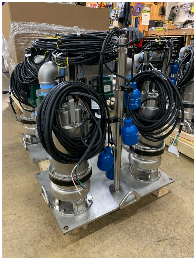
Sump pump package with two Ebara® Dominator stainless steel submersible sewage pumps, fabricated steel mounting/lifting plate, and float switches for drop-in installation in a drainage sump
