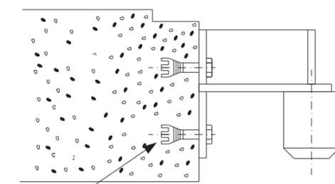
Hole-in anchor bolt Fig. 3
