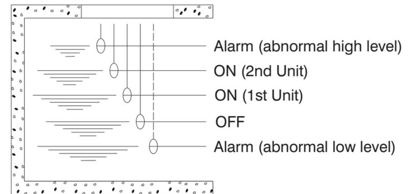
Fig. 17 Two-Unit Alternating Operation
