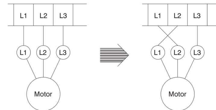
Fig. 19 Change of Connections for Normal Pump Performance
