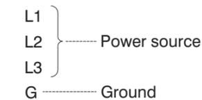
**⚠ WARNING:** WHEN PREPARING POWER CABLE LEADS FOR CONNECTION TO CONTROL, IT IS ESSENTIAL THAT THE GROUND LEAD BE LONGER THAN THE POWER LEADS. THE GROUND LEAD MUST HAVE AT LEAST 2" (50 MM) SLACK REMAINING AFTER CONNECTION, WHEN SPACE PERMITS. THIS IS DONE FOR ELECTRICAL SAFETY. IF THE CABLES IS MISTAKENLY PULLED OUT, THE GROUND LEAD WILL BE THE LAST WIRE BROKEN.
